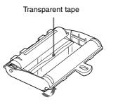
Turn the spools in the direction of the arrow to remove any slack until the transparent tape cannot be seen.
