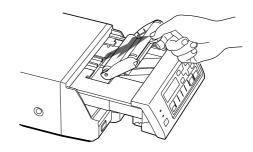
**3** Remove any slack from the ink ribbon. Wind the spools in the direction of the arrow until the start position marker appears as illustrated.
